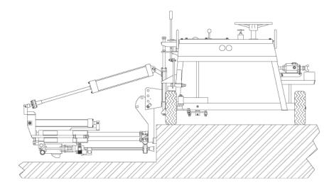
Three position drilling with 48" unit: Horizontal, Vertical and 35 degree stitch Urethane filled tires 3-1 skew drilling standard Adjustable drill height and depth Dust collection is available
