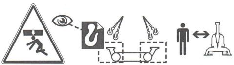
Risk of compression or crushing injury. Locate and attach the lifting equipment to all the lifting eyes. Keep your distance Ensure that the weight is evenly distributed when lifting. Lift slowly and cautiously. If the machine has a tendency to lean, use another lift or change the position of the arm system.
