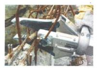
The HCS 6 **C** is specially designed to expand and separate material, e.g. ripping radiators or door frames from walls or breaking up concrete pieces. The tool has a shear set for cutting-up various materials, like reinforcements up to 20 mm (0,8 inches) in diameter.
