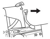
Loosen the drive gear. Use a spanner as a counterhold. (The combination spanner or bearing tool can be used as a counterhold.)
