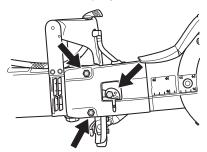
Turn the eccentric plate anti-clockwise with a screwdriver or a torx driver. This tightens the drive belt by pushing the bar forwards.
