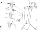
lashing devices. Only use load carrying devices and lifting gear and with sufficient lifting capacity (observe the operating weight of the machine). Lift the machine only by the attached transport eyelet (Pos.1).
