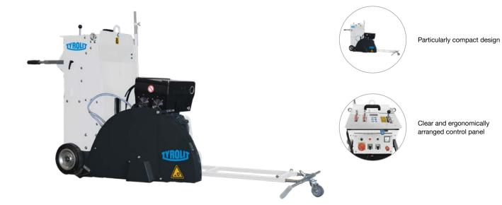
The robust, powerful floor saw FSE1022 was specially developed for cutting tasks in buildings. The frequency converter enables the continuously variable adjustment of the cutting shaft speed, making it possible to set the optimum cutting speed for every saw blade diameter. The low centre of gravity and precise distribution of weight on the axes ensure stability and excellent directional stability.
