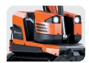
**PROTECTION OF VITAL PARTS** The electric motor, hoses and cables are protected by the robust lower chassis.
