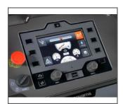
**TRACKING FOR STRAIGHT CUTS**Electric tracking system includes position indicator on the display, it can automatically return to neutral position and has the ability to memorise last used setting.
