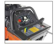
**CONTROL PANEL**All important functions are easy to reach and monitor, such as; blade rpm, forward speed, electronic tracking, depth gauge, belt and pulley ratios, runtime and service minder.
